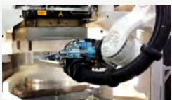
Release agent spraying and/or mold cleaning
